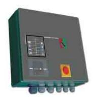
Kaeser offers an enhanced starter control panel to monitor and regulate booster operation. Units from 3 to 25 hp are 230/460 V with direct on-line start. Units 30 hp and larger are 460 V with wye-delta start (consult factory for other voltages). The starter is designed to be wall-mounted.
